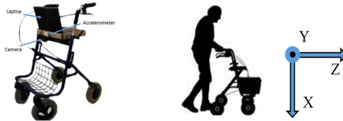
Fig. 1. (a) Hardware setup; (b) Accelerometer axis configuration.
